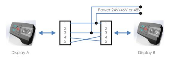
Setp 3 :Power on display A or display B , some guide message will show on screen, do it as the guide. Setp 4: Long press DOWN button will receive settings from other , Long press UP will send settings to other
